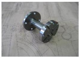
Cardan shafts differ in every car owing to the positioning of the gearbox and the engine. Gentry Restorations can manufacture one specifically for your car at one set cost. Contact us for more details and advice.
